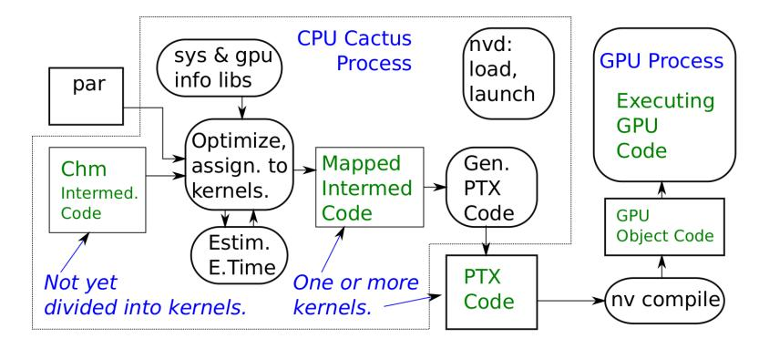
Calculation dynamically mapped to kernels based on app and sys params.
