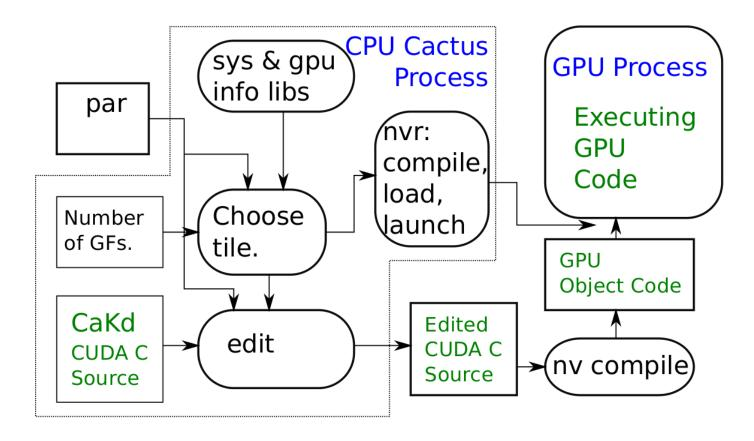
Tile sizes chosen dynamically, based on system and application parameters.
